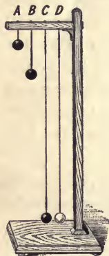
FIG. 42. — Pendulums of Different Lengths and Masses.
